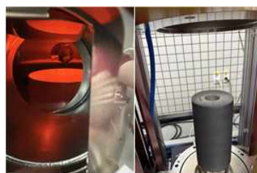
Figure 1. A soil heating reactor system at KIGAM
